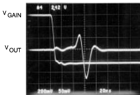
V_{GAIN} Overload Recovery Response—No AC Input
